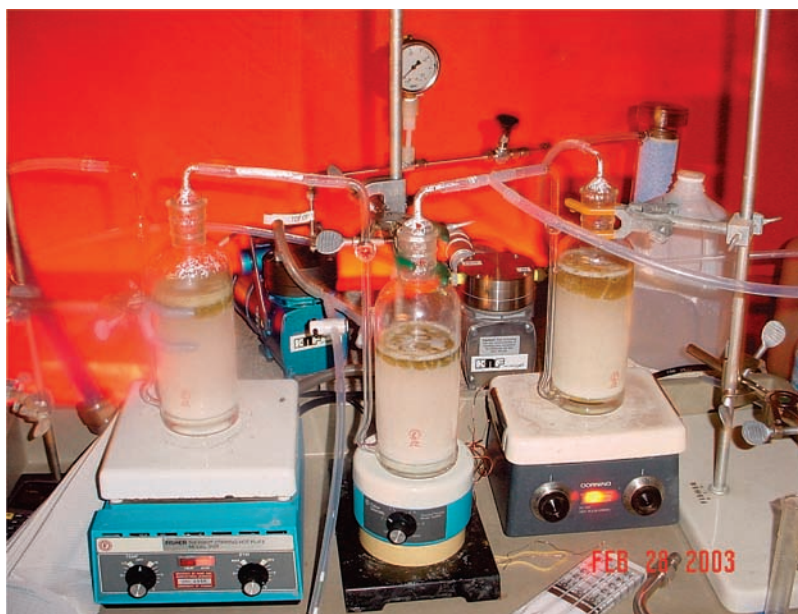
Figure 2. Gas sampling apparatus used to destroy methyl bromide from a slipstream of methyl bromide.
